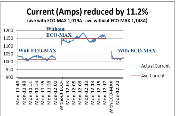
The graph above shows the reduction in current of 11.2% with the ECO-MAX in operation. This equates to a 9% reduction in total power drawn from the network (see graph below), delivering both environmental and financial benefits to Viridor.
