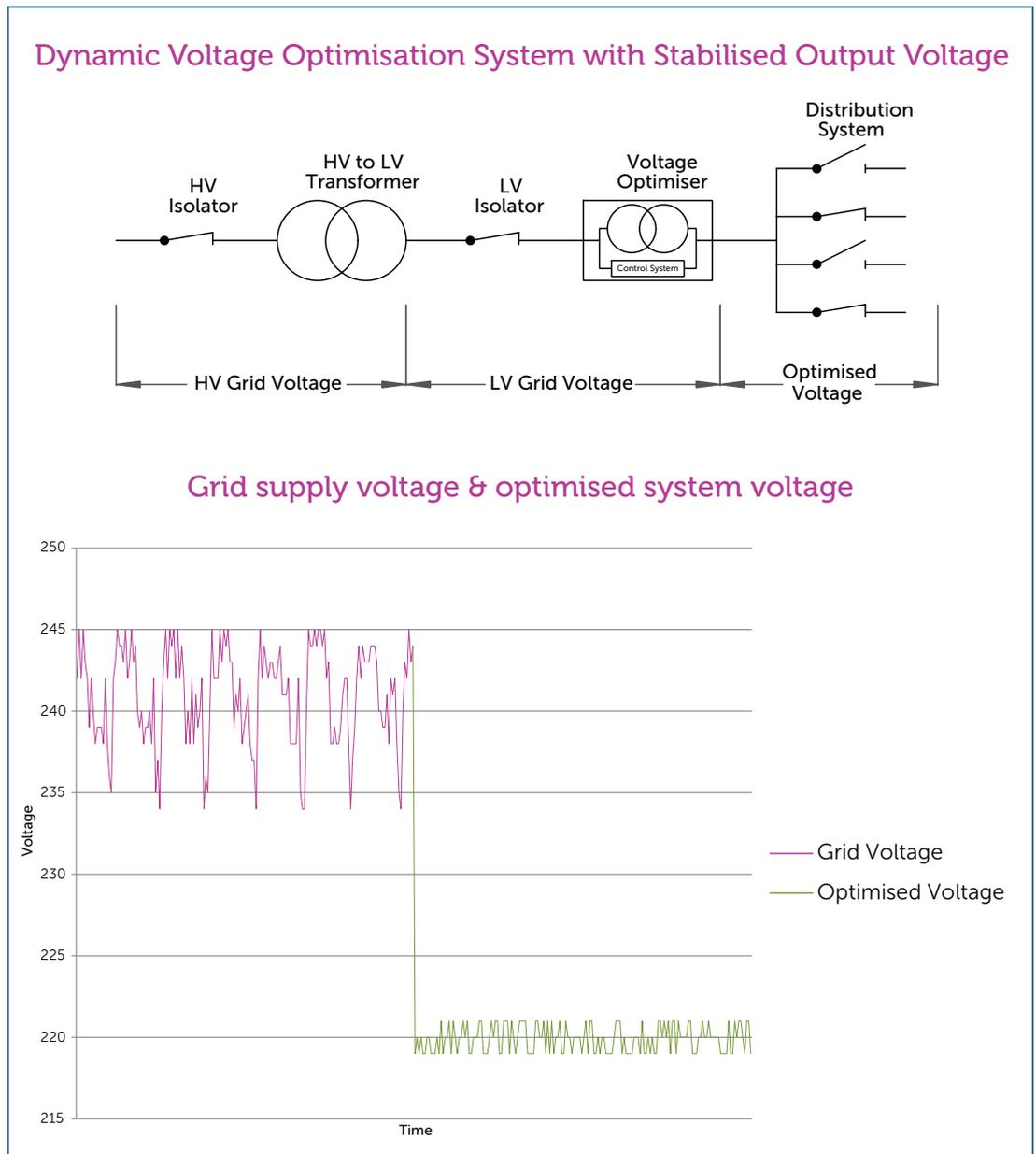
FIGURE 5: RESULT OF DYNAMIC VOLTAGE OPTIMISATION WITH A VARIABLE REDUCTION TO ACHIEVE A STABLE OPTIMISED VOLTAGE
