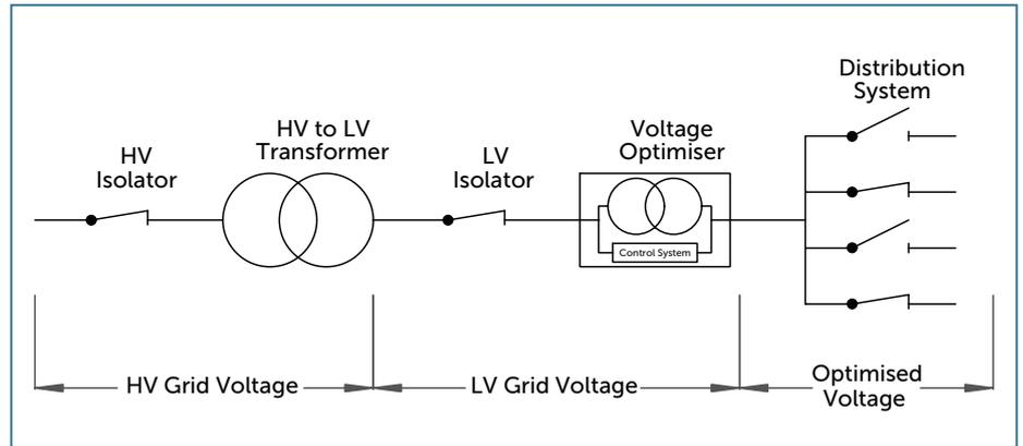
FIGURE 1: TYPICAL VOLTAGE OPTIMISATION INSTALLATION
