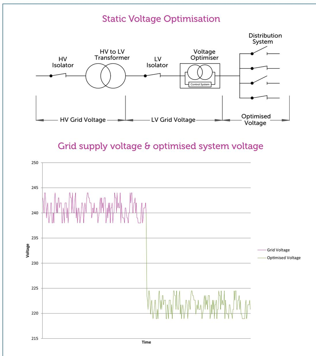
FIGURE 3: RESULT OF STATIC VOLTAGE OPTIMISATION WITH FIXED 8% REDUCTION
